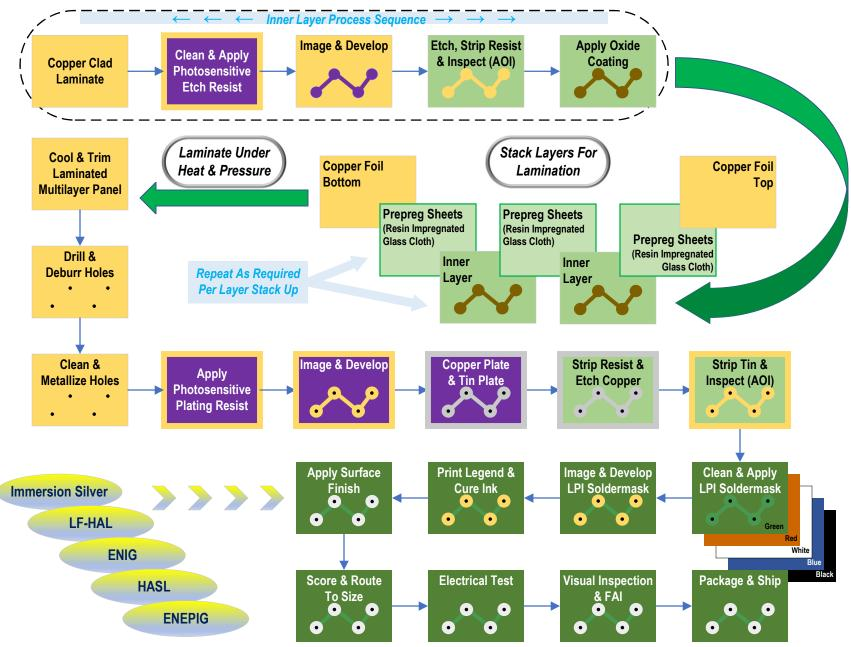
Blind Vias, Buried Vias, Filled Vias and other higher technologies use these same processes in differing sequences and may be augmented by additional specialty processes such as Planerization, Laser Drilling, Controlled Depth Drilling, etc. Double Sided boards begin at **Copper Clad Laminate** followed by **Drill & Deburr Holes**.
